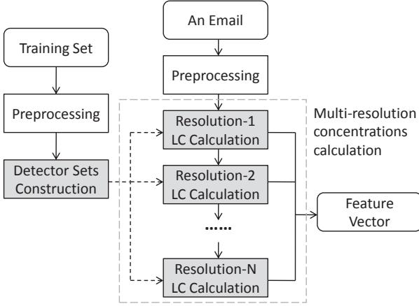
Fig. 1. The structure of MRC model
